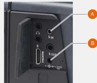
Flash Sync and Power Connections
